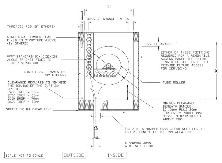
N.B THE INTERNAL END OF THE BULKHEAD MUST BE CLEAR TO AT LEAST THE BACK OF THE GUIDE OR OVERALL THE REMOVABLE SIDE MULLION
