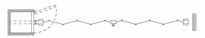
Single stack with "S" curve into pocket using 2 x 1 35° curves
