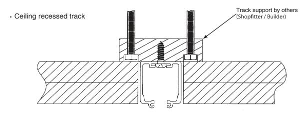
NOTE: It is unacceptable to have any gap between the track and the track support.
