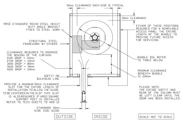
N.B THE INTERNAL END OF THE BULKHEAD MUST BE CLEAR TO AT LEAST A MINIMUM  $50\,\mathrm{mm}$
