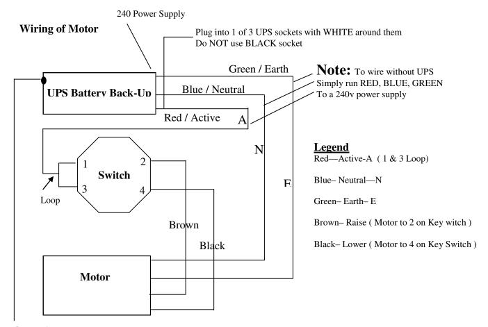
IMPORTANT To commission UPS—push "On button" on top front of unit, one beep should sound. Push same button again and hold in till "2 beeps" are sounded—the unit should now be in UPS mode
